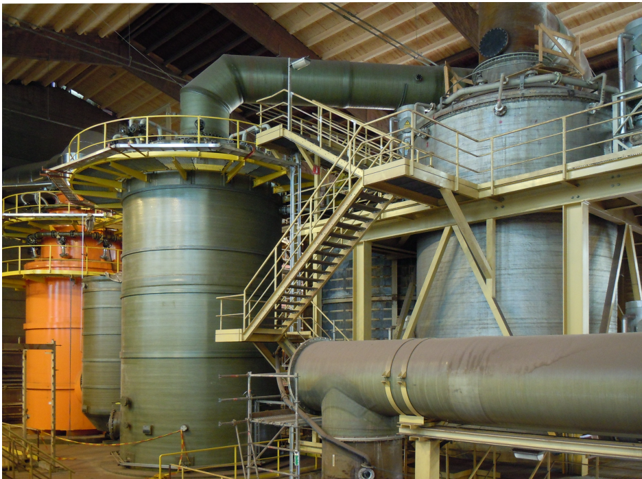
Pic. 5: Complex multistage wet scrubbing unit installed at a metallurgical plant.
