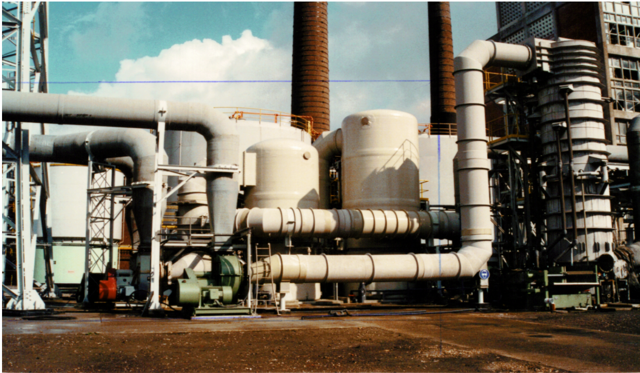
Pic. 6: Scrubbing plant for the absorption of noxious gas components and the removal of acidic mists and salt aerosols downstream of multiple-hearth furnaces for the production of inorganic raw chemicals
