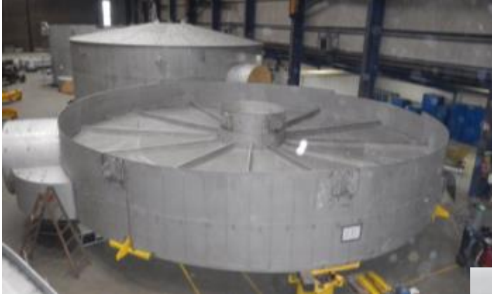
Figure 8: Segment of a Grembrane Converter in the workshop
