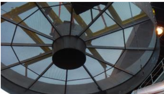
Figure 10: Tray element under assembly
