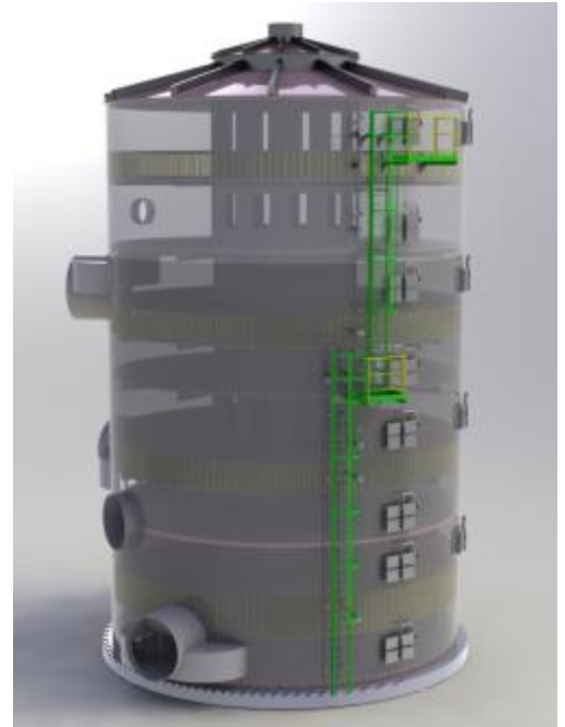
Figure 2: 3D-Modell of a Grembane-Converter
