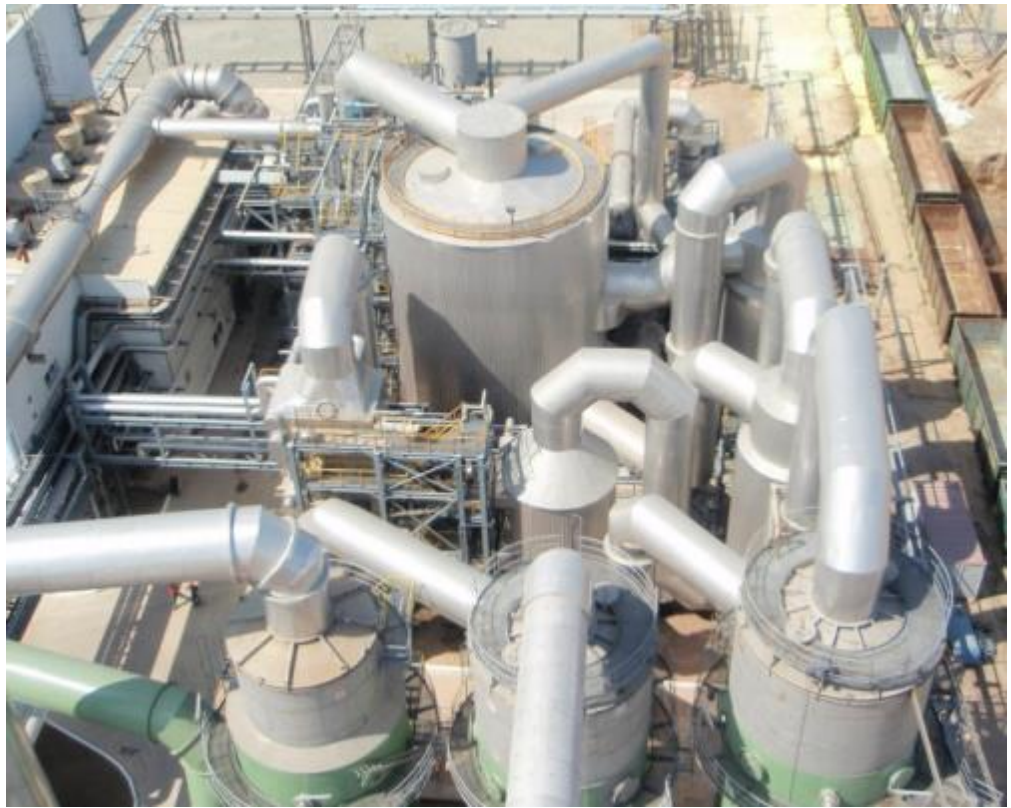
Figure 15: 1,800 tpd Mh Sulphur Burning Plant
